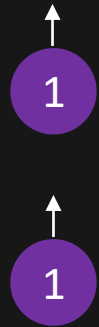
Measuring the value of one qubit breaks the entanglement and collapses both the qubits
